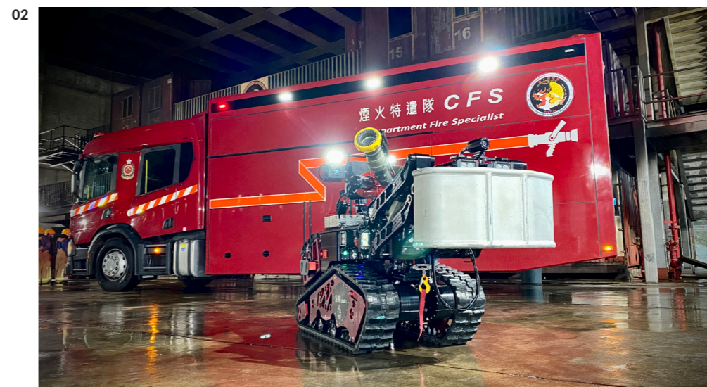
01 灭火机械人的模组化设计可让其改装成不同模式执行工作。 02 The modular design of the firefighting robots offers interconvertibility that allows them to work in different modes.
