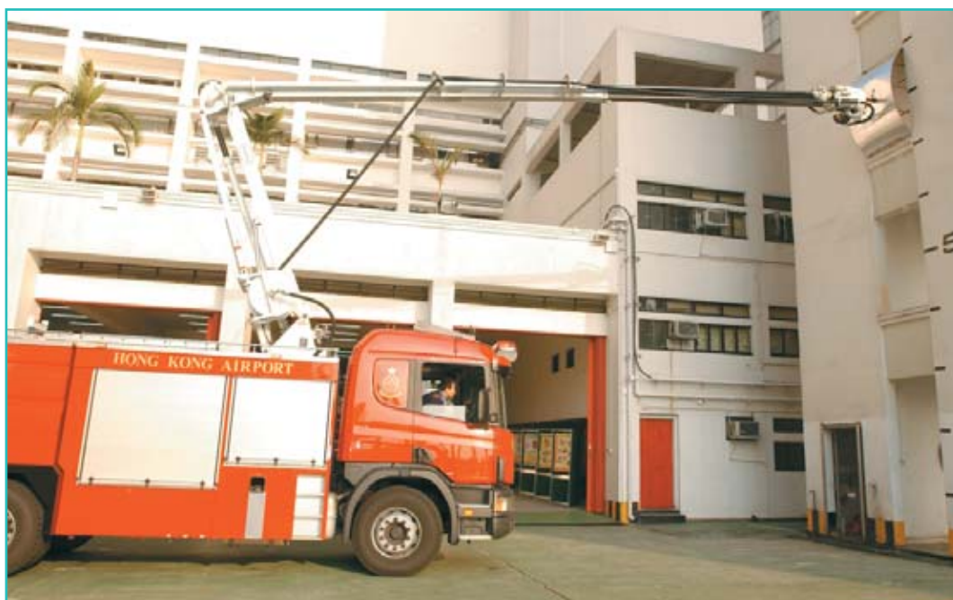
◀ 無積升降台裝設刺針噴管 Jackless Snorkel equipped with piercing nozzle
