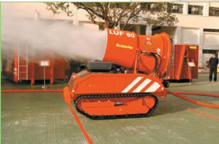
◀ 流动灭火支援车专用于隧道火警 Mobile Fire-fighting Supporting Machine designed for tunnel fires
