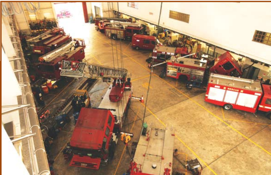
消防處工程部負責保養及維修消防車輛 F.S. Workshops provide maintenance and repairs to fire appliances
