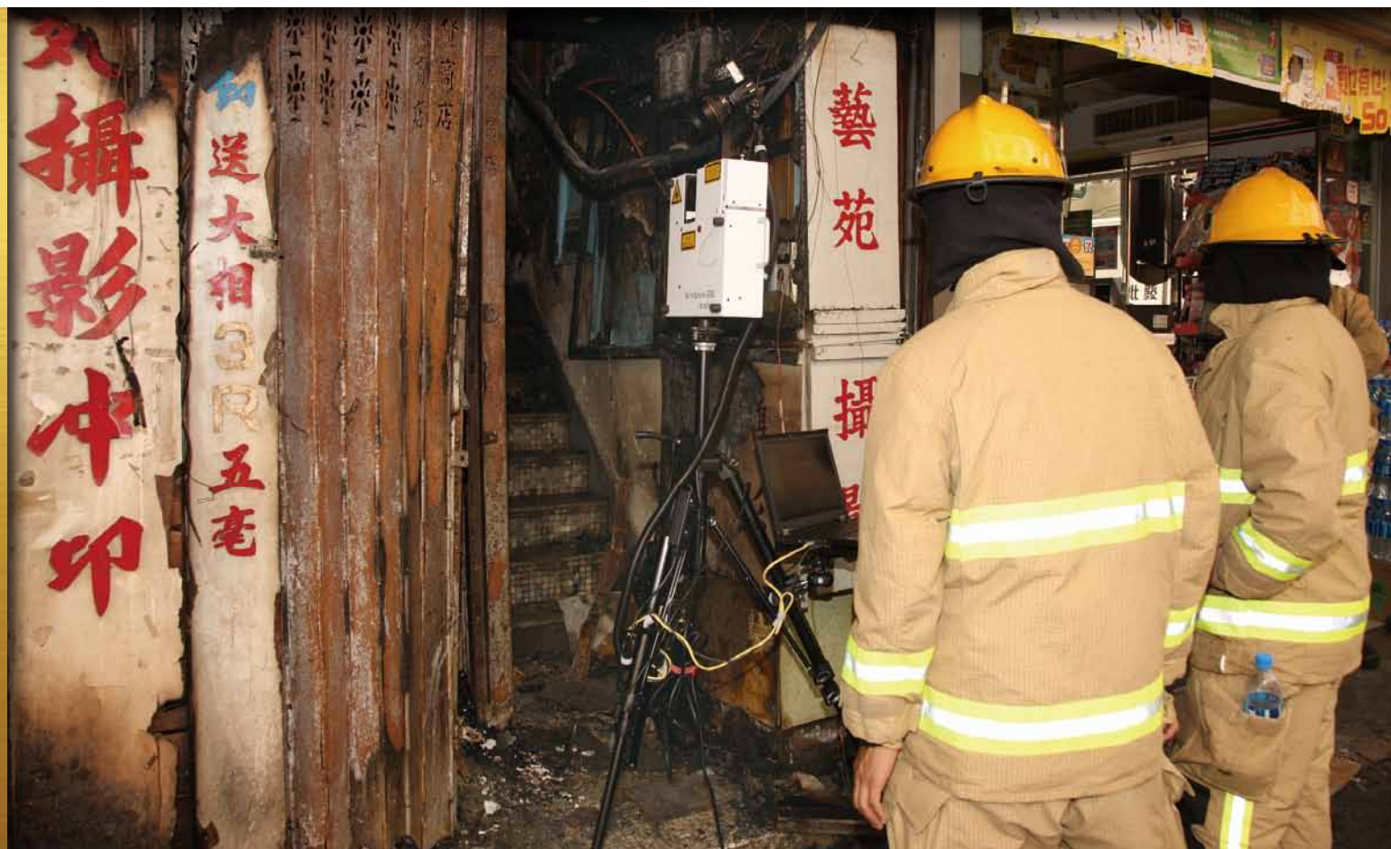
火警調查組成員使用目前最先進的火場案情重組分析工具「三維場景激光掃描儀」，以協助調查火警起因 Members of Fire Investigation Group use the Deltasphere 3000 IR 3D Scene Digitizer, which is today's most advanced analysis tool on fire scene reconstruction, to assist their investigations into the cause of a fire
