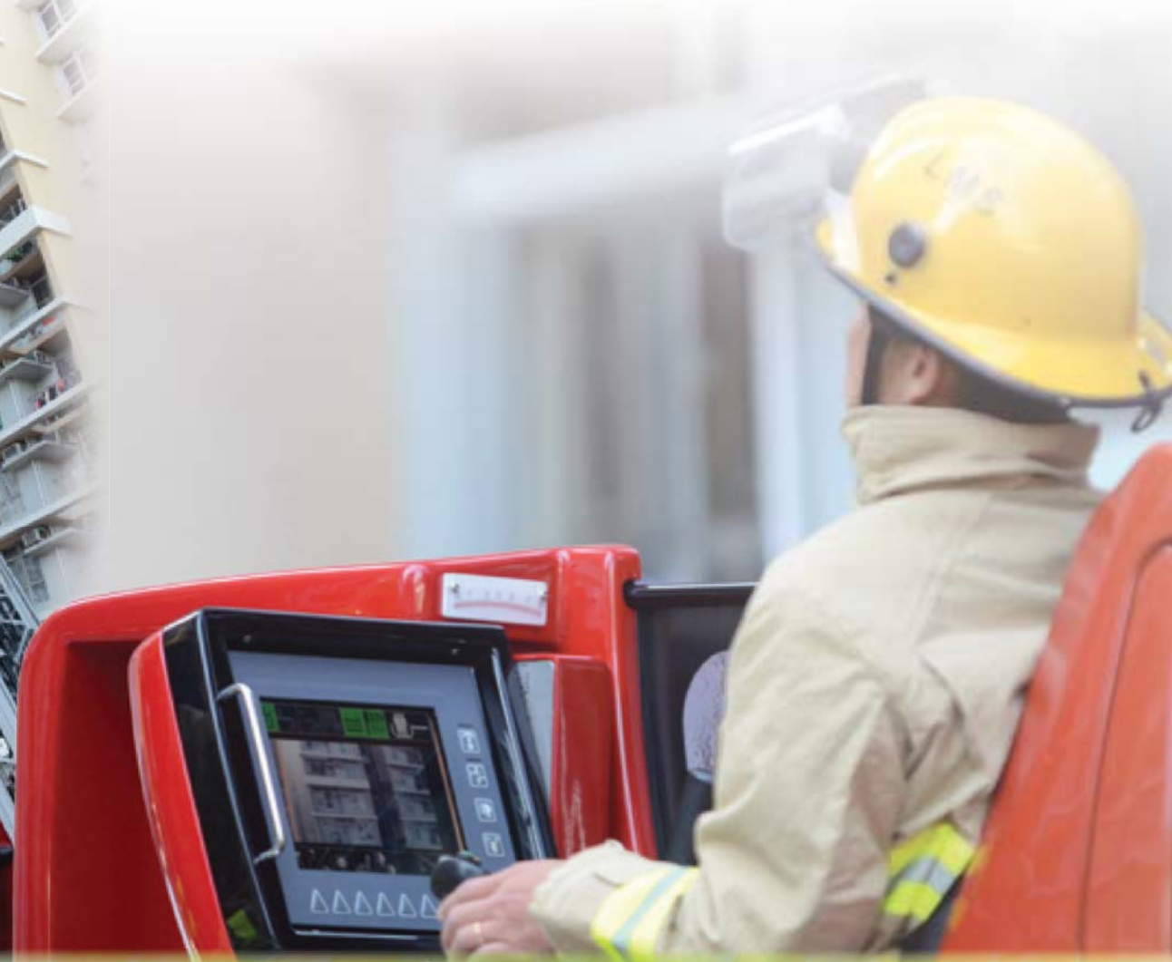
视像镜头将影像传送到 55 米钢梯车上的屏幕（头条日报图片） The image captured by a video camera was shown on the screen on the 55-metre turntable ladder (Headline Daily photo)
