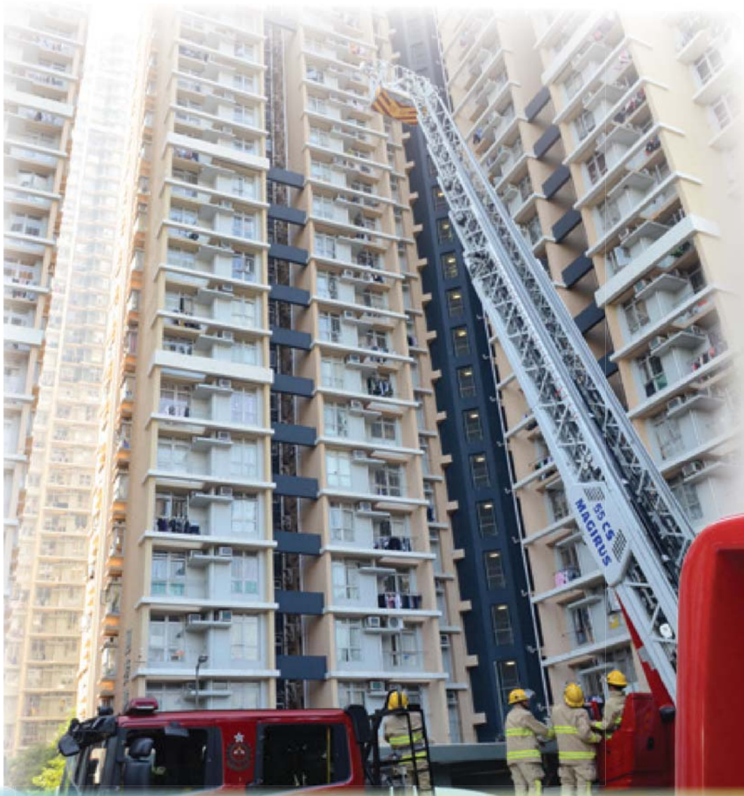
55 米钢梯车设置不具录影功能的视像镜头，有助消防人员了解现场环境，以采取适当的救援行动（星岛日报图片） The 55-metre turntable ladder is equipped with a video camera (with no recording function) to facilitate fire personnel in assessing the situation at scene before carrying out rescue operation (Sing Tao Daily photo)
