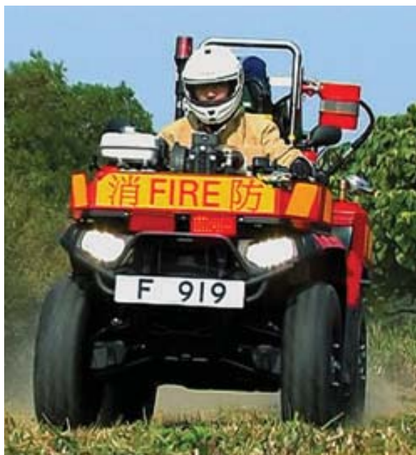
迷你消防车可于郊区狭窄而崎岖的路面行驶，展开灭火救援行动 The Mini Fire Truck can travel on narrow and rugged roads in suburban areas to carry out firefighting and rescue operations
