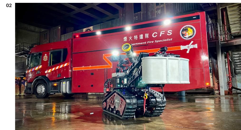
01 滅火機械人的模組化設計可 02 讓其改裝成不同模式執行工作。 The modular design of the firefighting robots offers interconvertibility that allows them to work in different modes.
