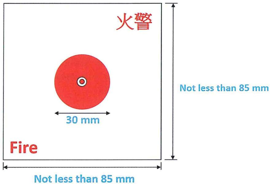
Figure 3 – For Detector inside Lockable Rooms
