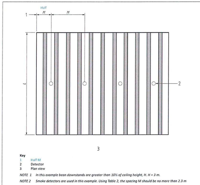
Figure 11 c) – Ceilings : Cells formed from joists [see 22.3k) and 22.3l)]
