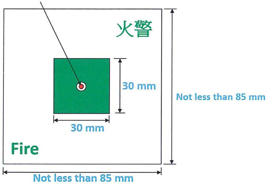
Figure 1 – For Detectors inside Floor Voids
