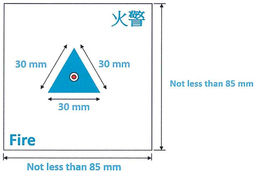
Figure 2 – For Detectors inside Ceiling Voids
