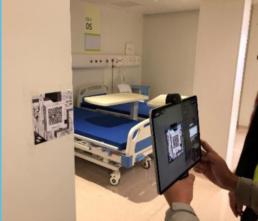
QR Code was equipped at Ward for access of Building Information Modelling (BIM) data
