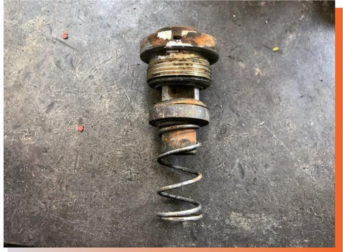
Moving parts of Pressure Reducing Valve
