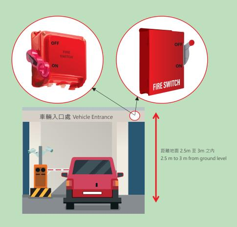
\*備註:以上圖片僅供參考。開關掣的規定詳載於消防處通函第 4/2020 號的附錄 Remarks: The above pictures are for reference only. Details of the switch are provided in the Appendix of FSD Circular Letter No. 4/2020
