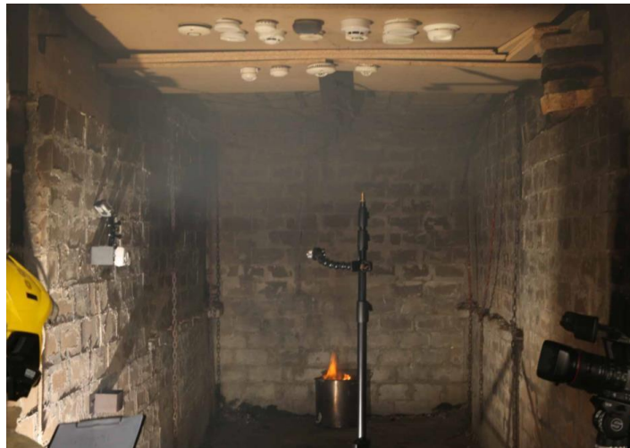
Figure 4 – In-house testing of various stand-alone fire detectors
