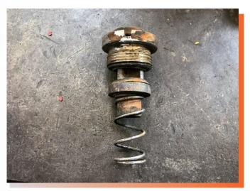
Moving parts of Pressure Reducing Valve
